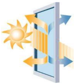
LOW E COATING AND GASSES MANAGE VISIBLE LIGHT AND HEAT TRANSFER
