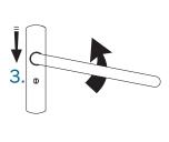
As the handle is turned up, door is starting to lower to rest on the track.
